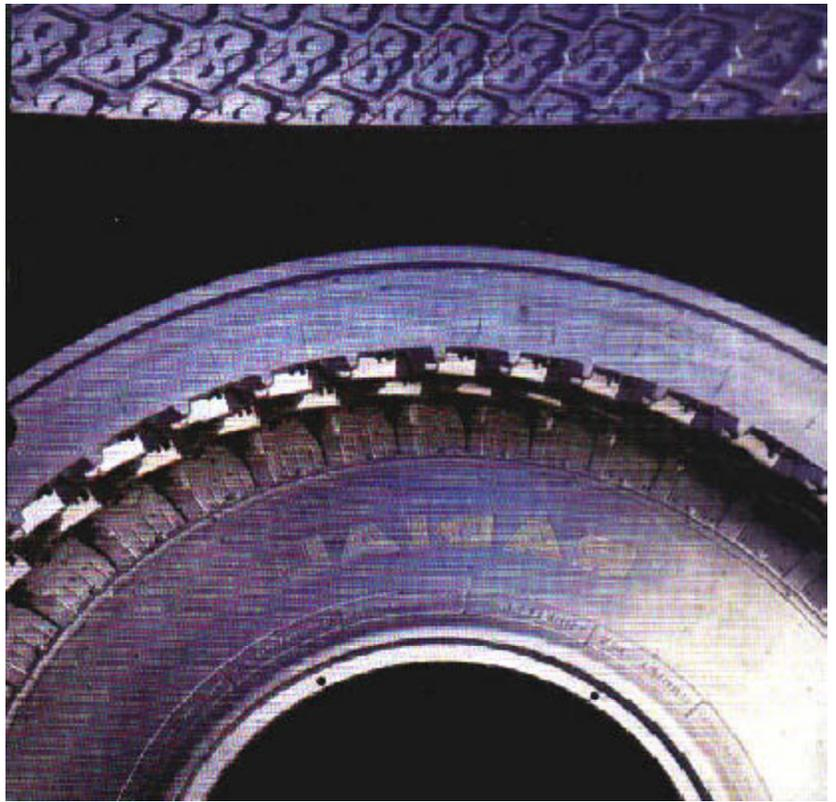
CO<sub>2</sub> blasting has had a big impact on tire mold maintenance. Strengths include in-press cleaning and simultaneous microvent clearance.
