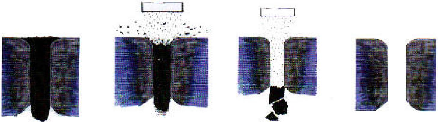
small amount of metal from the mold surface, and by imparting a much 'rougher' (more micropeaks and valleys) surface finish into the mold from the chiseling effect of thousands of abrasive impacts. The rough surface creates an 'anchor pattern' that was not present in the original mold surface.
