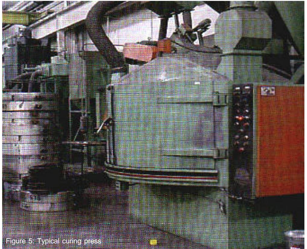
Figure 5: Typical curing press
